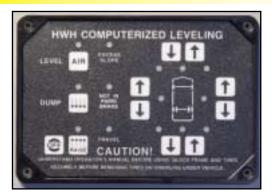
The HWH Air Leveling System features computer (touch panel) control and our HWH Leveleze Indicator Light System. The control pad can be dash mounted for operator convenience.
