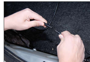
Connect wire from main bracket to the wire coming from the monitor
